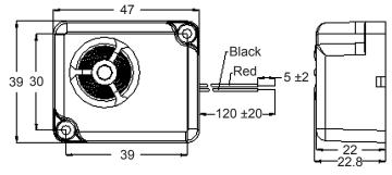
Dimensions : Millimetres Tolerance: ±0.5mm
