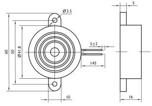
Dimensions : Millimetres Tolerance: ±0.5mm
