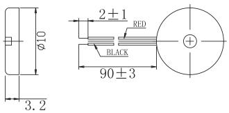
Dimensions : Millimetres Tolerance: ±0.5mm
