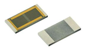
PCAN series chip resistors are designed on aluminum nitride ceramic substrates with enlarged backside terminations to reduce the thermal resistance between the topside resistor layer and the solder joint on the end users circuit assembly.
