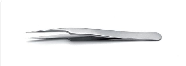
5A.SA Tips: straight, extra fine, superior finish. OAL: 115mm
