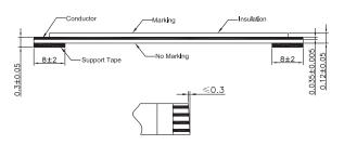
Dimensions: Millimetres Tolerances: ±0.3mm
