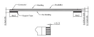
Dimensions: Millimetres Tolerances: ±0.3mm
