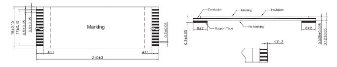
Dimensions : Millimetres Tolerances: ±0.3mm
