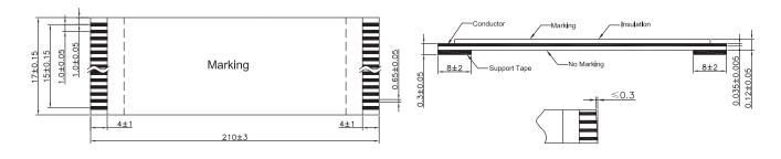
Dimensions : Millimetres Tolerances: ±0.3mm
