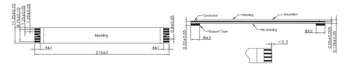
Dimensions: Millimetres Tolerances: ±0.3mm
