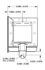
Solenoid shown energized in drawing with plunger fully seated
