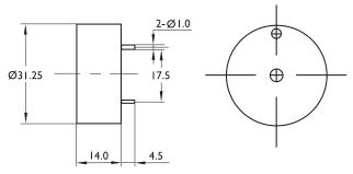
Dimensions: Millimetres Tolerance: ±0.5mm
