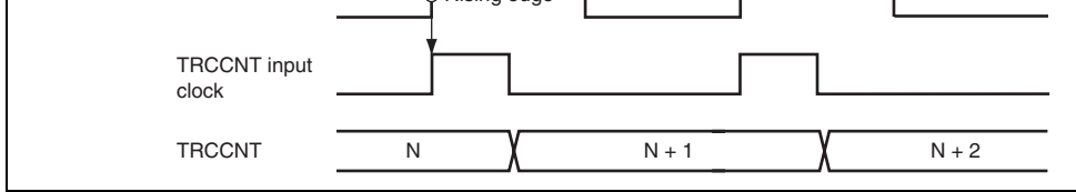
Figure 13.23 Count Timing for Internal Clock Source
