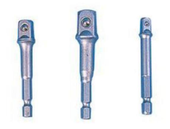
Hardcase Power Extension Bit Set, Features: A set of 3 extension bits taking a 1/4 hexagonal screwdriver fitting and extending to a 1/4, 3/8 and 1/2 square drives, Length: (Extension Bar) 2 1/2. Use any power driver with 1/4", 3/8", and 1/2" sockets.
