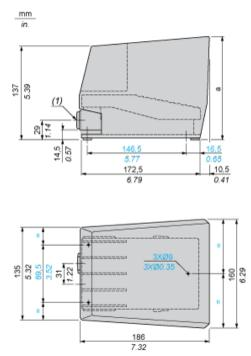
(1) 2 tapped entries for  $n^{\circ}$  16 (Pg 16) cable gland. For ISO M20, use adaptor DE9RA620.
