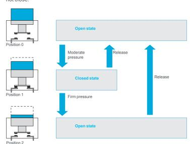
Operating principle of an enabling switch
