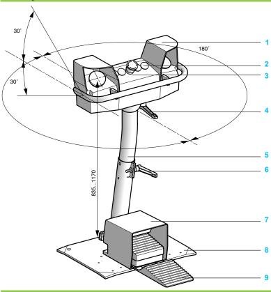
The control station 1 has five cut-outs (Ø 22 mm) 2 as standard. Five additional cut-outs are possible 3. Its pedestal 5 enables the following quick and simple adjustments:
