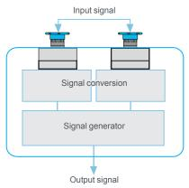
Functions of a two-hand control station
