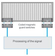
Functions of coded magnetic guard switches
