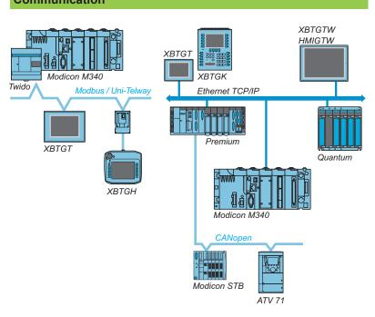
Magelis Standard Advanced panel communicate with PLCs via one or two integrated serial links, using communication protocols:
