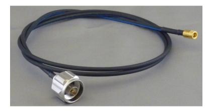
The 112A cable is designed to connect the 100 series probes to spectrum analyzers or other instruments with Type N connectors. This double-shielded cable has good RF performance from DC to 6 GHz. Its narrow diameter gives the 112A cable high flexiblity, making it convenient and kink-free when using the probes manually.
