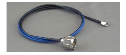
The 114A cable is designed to connect the 150A EMC probe amplifier to spectrum analyzers or other instruments with Type N connectors. This double-shielded cable has good RF performance from DC to 6 GHz. One end of the cable has a male SMA connector to connect to the amplifier, and the other end is a male Type N connector. This allows it to connect to spectrum analyzers or other equipment with female Type N connectors.
