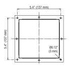
Drilling template for mounting frame
