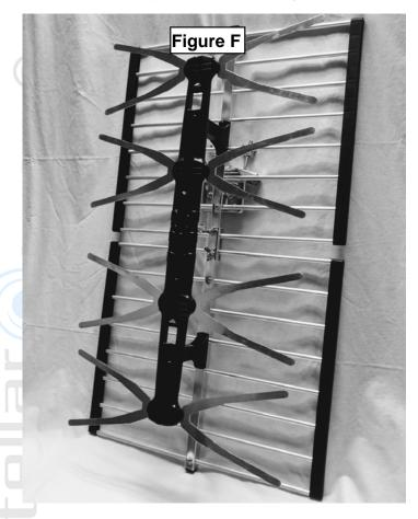
**Step 6:** Connect the provided coaxial cable to the F connector on the center of the array assembly.
