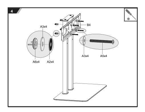
Determine the optimum height on the rear pedestal to attached the (B4) bracket. The best method to do this is to measure from the center of your television screen to the bottom most edge of the TV set. This will tell you the minimum clearance needed on this Universal Base.
