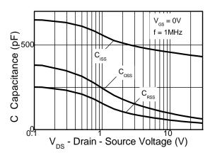
Capacitance v Drain-Source Voltage
