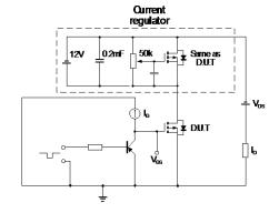
Gate charge test circuit
