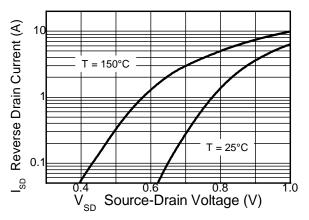
Source-Drain Diode Forward Voltage
