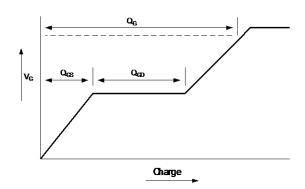
Basic gate charge waveform
