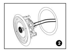
Connect the speaker wires to the speaker.
