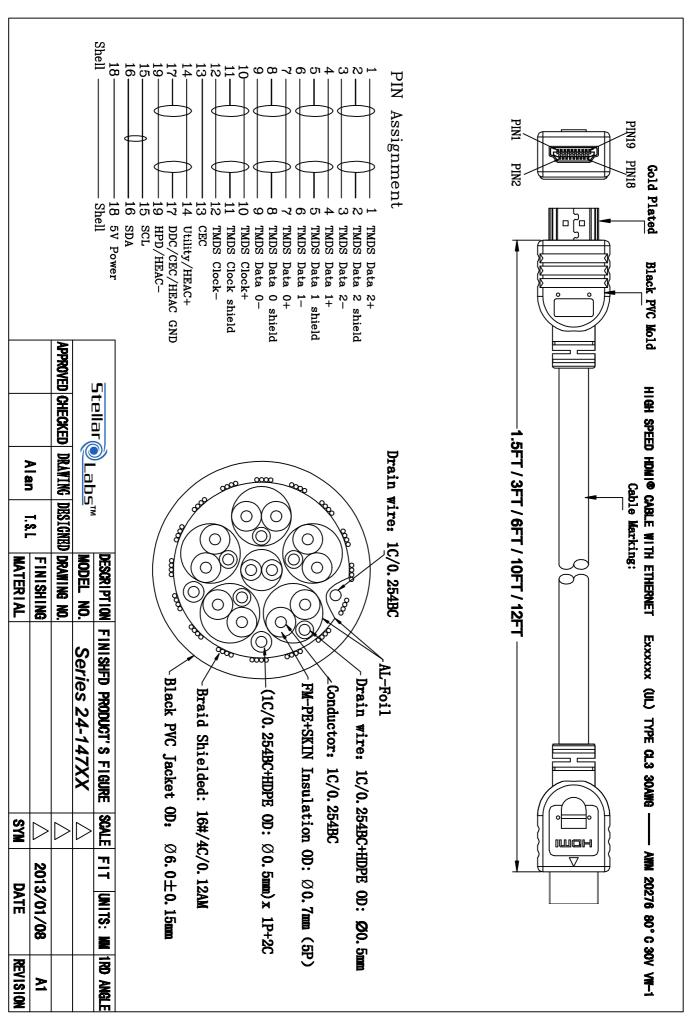
Stellar Labs High Speed HDMI Cable w/Ethernet www.mcmelectronics.com
