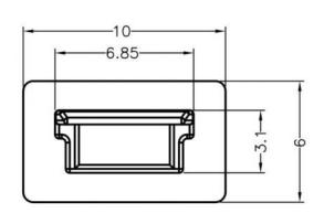
All measurement does not include gate which raises under 1.2mm.
