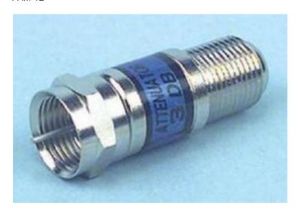
Nickel-plated, solid brass body, monolithic ceramic printed circuit board, ensuring rugged construction, etched glaze-type resistors provide ±5% accuracy and excellent return loss, small 1.375" size, 22-gauge spring steel center pin, female to male fitting, not DC passive.
