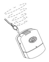
To activate both Mugger Stopper Plus alarm and strobe light, simply pull out plug on top of unit.
