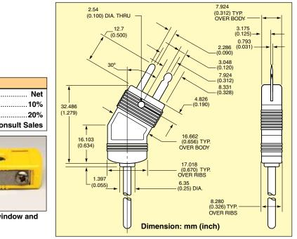
Connector blades are stamped with thermocouple alloy
