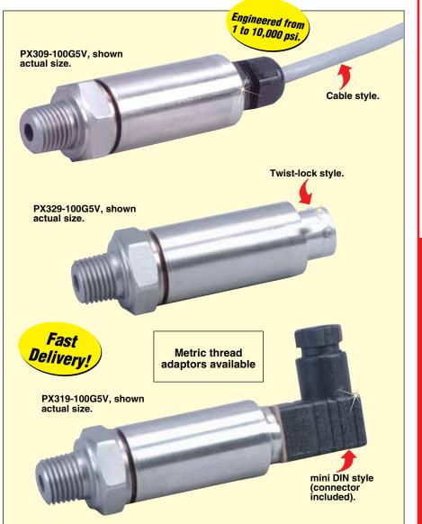
Burst Pressure: 5x capacity or 25 psi, whichever is greater Response Time: <1 ms Shock: 50 g, 11 ms half-sine shock Vibration: ±20 g Wetted Parts: 316 SS for all psia ranges and 1 to 50 psig; 17-4 PH SS for ranges 100 to 10,000 psig Pressure Port: ¼-18 MNPT **Electrical Connections:**
