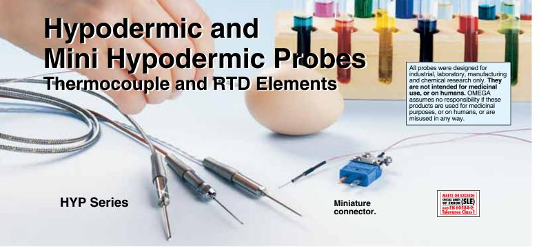
OMEGA® Hypodermic Needle Temperature Probes are designed for industrial, laboratory, manufacturing and chemical research applications. Five probe types are available, with diameters from 0.2 to 1.65 mm (0.008 to 0.065"). The HYP0, HYP1 and HYP2 have type T (Copper-Constantan) thermocouple elements, while the HYP3 is available in J, K, T or E calibration, and the HYP4 has a 100  $\Omega$  Platinum RTD (a = 0.00385).
