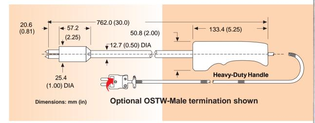
Specifically designed for use where surface temperatures reach up to 1260°C (2300°F) and rough handling is routine, OMEGA's foundry probe uses large, heavy duty tips that can penetrate surface slag to measure the true temperature of the casting. The surface to be measured must be electrically conductive. The lead wires are 16-gage stranded wire with high temperature insulation and stainless steel overbraiding for added protection.
