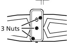
6. Place the bottom of the middle section on the middle section top. Make sure to line up with the pegs at the top and the holes with the screws.
