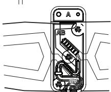
5. Place the holes of the second wing over top of lower left and middle screws. The wings will slightly overlap. The AB printed on the wing should appear at the lower right (upside down).
