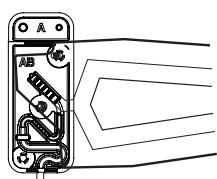
4. Place the holes of one of the wing sections over top right and middle screws. The letters AB printed on the wing should be visible in the upper left corner of the wing.
