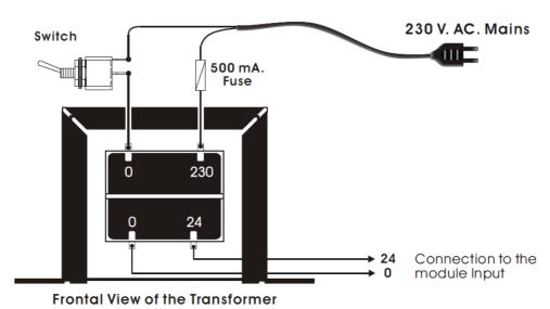
Connect both cables from the mains input (230 V A.C) to the superior terminals indicated as 0 & 230. (See the General Wiring Map).
