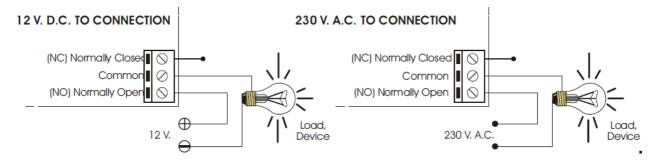
**INFORMATION ABOUT THE OUTPUT.** During the operating mode and according to its load, it could happen a fluctuation or an incorrect working of the output. In such case, you have to install an anti-spark circuit between both contacts of the relay used in this connection, as it is indicated on the drawing.
