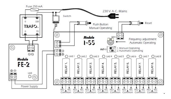
**OUTPUT. CONNECTION OF THE LOAD.** The output Module (I-55) is controlled by a relay, allowing any load until 5 A. as maximumconsumption. The relay has 3 output terminals the normally open at quiescent (NA), the normally closed at quiescent (NC) and the common. The operating of this mechanismis the same as a switch with two (2) terminals NA and common, if you wish that the output will be activated during the timer, or between the NC and the common to obtain the reverse operating.
