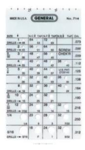
The #714 Screw Thread Gage quickly identifies thread pitch, tap size and drill bit size for machine and wood screws, bolts and common rivets and cotter pins up to 5/16 in. across
