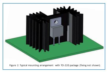
The package should be fitted to the heatsink using a suitable thermal interface material, for example a thermal pad or paste such as Dow Corning DC340. It should be secured with an M3 mounting screw tightened to give void-free thermal contact and to a maximum torque of 0.9Nm.
