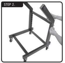
2. Line up all three cross bars with other side and hand tighten large screws with washers. After all three bars have been attached use an allen wrench to finish tightening.
