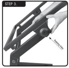
Attach top rack to assembled rack by lining up rotating links over each other. Start with one side and snap the other into place.
