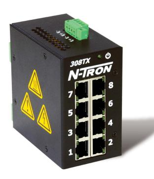
The 308TX simplifies plant wiring by eliminating the need to bring data acquisition and control network connections back to a climate controlled environment. The 308TX has extended operating environmental specifications to meet the harsh needs of the industrial environment. For cost savings and convenience the network switch can be DIN-RAIL mounted alongside Ethernet I/O or other Industrial Equipment.
