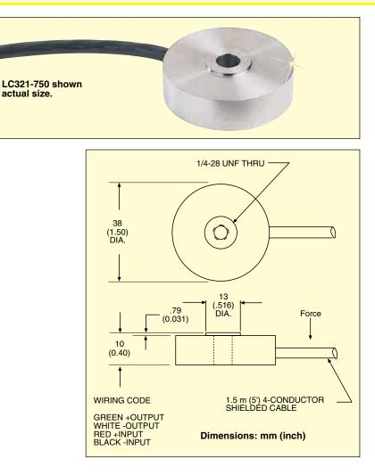
Safe Overload: 150% of capacity Ultimate Overload: 300% of capacity Input Resistance: 360  $\Omega$  minimum Output Resistance: 350 ±5  $\Omega$  **Construction:** Stainless steel **Electrical:** 1.5 m (5') 4-conductor shielded cable
