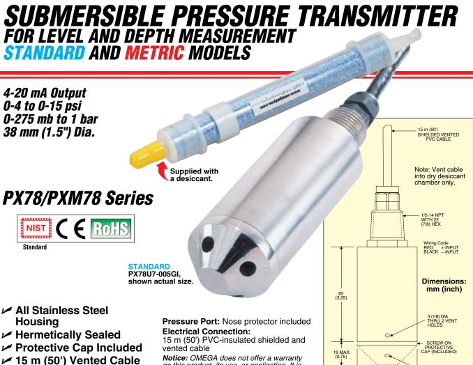
OMEGA's PX78/PXM78 are submersible transmitter suitable for liquid level and depth measurement. Their all stainless steel, hermetically sealed housing makes them suitable for immersion in most industrial liquids and oils. A 15 m (50') vented cable (longer lengths available) provides an atmospheric pressure reference.
