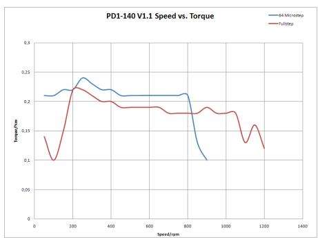
Figure 7.1: PD1-140-42-SE torque curve
