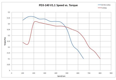
Figure 7.3: PD3-140-42-SE torque curve
