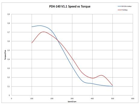
Figure 7.4: PD4-140-42-SE torque curve
