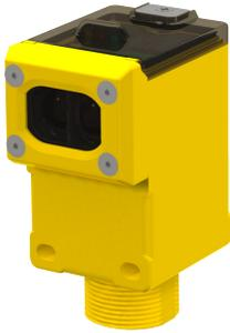
With a diffuse-mode sensor, the object is detected when the object reflects the sensor's transmitted light energy back to the sensor. No reflector or receiver is needed to detect objects.
