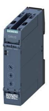
TIME RELAY, MULTI-FUNCTION, 2 CO CONTACTS, 27 FUNCTIONS, 7 TIME SETTING RANGE(1,3,10, 30, 100) (S, MIN, HR), AC/DC 12... 240V, AT AC 50/60HZ, LED, SCREW TERMINAL
