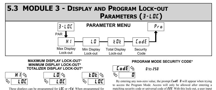
These displays can be programmed for LOC or rEd. When programmed for LOC, the display will not be shown when the DSP key is pressed regardless of Program Lock-out status. It is suggested to lock-out the display if it is not needed. The associated function will continue to operate even if its display is locked-out.
