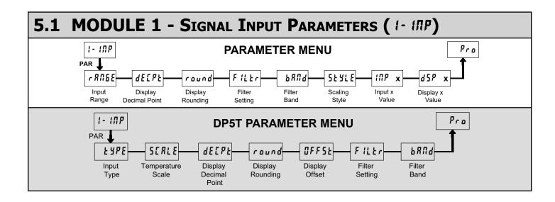
Refer to the appropriate Input Range for the selected meter. Use only one Input Range, then proceed to Display Decimal Point.
