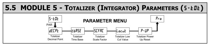
The totalizer accumulates (integrates) the Input Display value using one of two modes. The first is using a time base. This can be used to compute a timetemperature product. The second is through a user input or function key programmed for Batch (one time add on demand). This can be used to provide a readout of temperature integration, useful in curing and sterilization applications. If the Totalizer is not needed, its display can be locked-out and this module can be skipped during programming.
