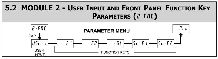
The user input is programmable to perform specific meter control functions. While in the Display Mode or Program Mode, the function is executed the instant the user input transitions to the active state.
