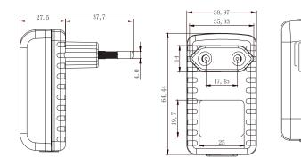
Dimensions : Millimetres Tolerance : ± 0.2mm
