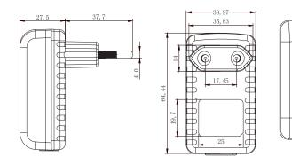
Dimensions : Millimetres Tolerance : ± 0.2mm
