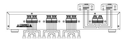
Insert your receiver/amplifier's positive (+) wires into the positive terminals, and negative (-) wires in the nagative terminals.
