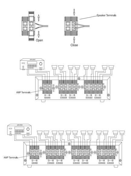
Press open the AMP terminals on the control center, then insert your receiver/amplifier's positive (+) wires into the positive (red) terminals, and negative (-) wires in the nagative terminals. Then press the tabs to close them.
