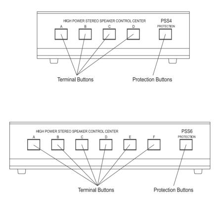
The control center lets you use one to four (PSS4) or six (PSS6) sets of speakers at a time, and is designed to operate with a stereo receiver/amplifier that has a maximum of 100 watts per channel, and with speaker systems that have a minimum impedance of 8 ohms (see "Impedance Chart" on page 5)
