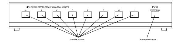
The control center lets you use one to eight sets of speakers at a time, and is designed to operate with a stereo receiver/amplifier that has a maximum of 100 watts per channel, and with speaker systems that have a minimum impedance of 8 ohms (see "Impedance Chart" on page 5)
