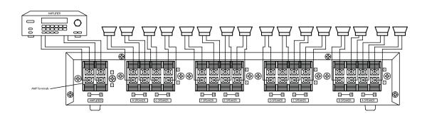
Press open the AMP terminals on the control center, then insert your receiver/amplifier's positive (+) wires into the positive (red) terminals, and negative (-) wires in the nagative (black) terminals. Then press the tabs to close them.
